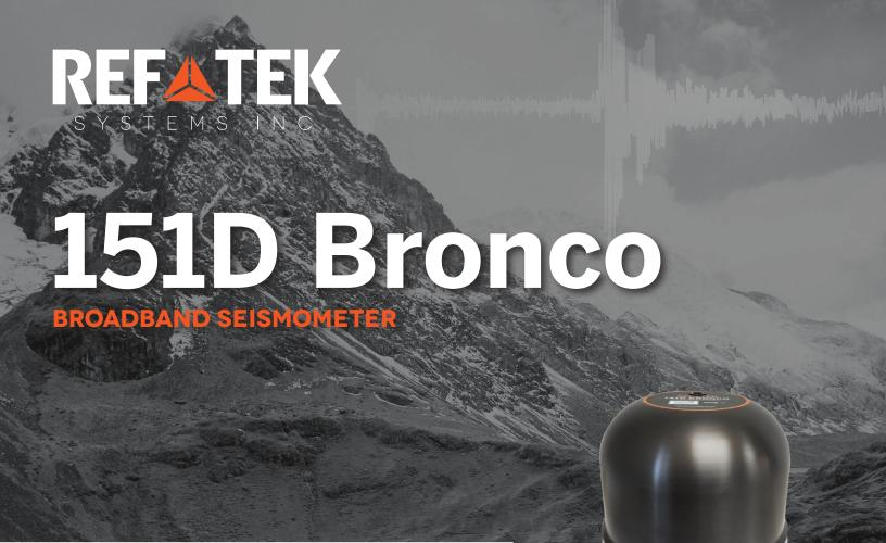
The 151D Bronco Broadband Seismometer is an observatory grade force-balance feedback velocity sensor available with the frequency bandwidth of 0.0083 Hz (120 sec) - 80 Hz. The seismometer contains three independent symmetrical sensors arranged in an orthogonal Galperin configuration. The sensor signals are deconvolved to provide the traditional ZNE orthogonal seismometer output for low noise and large dynamic range measurements.
